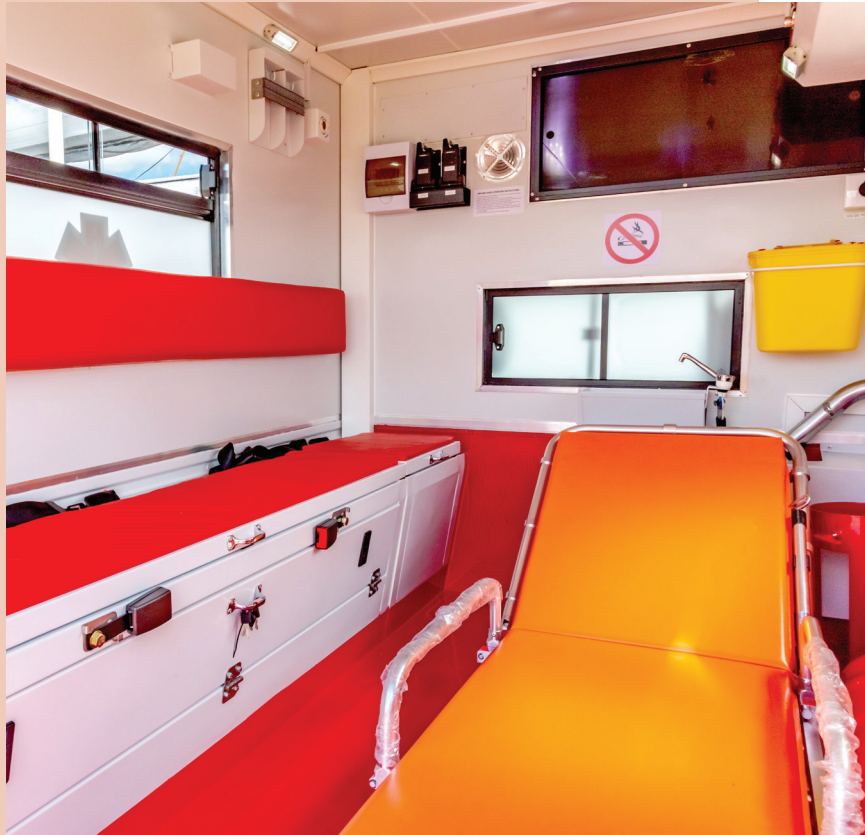
INTERIOR PATIENT CABIN FITTED WITH LIGHTING, SHOCK PROOF ANTI-SKID FLOORING, 12V POWER SUPPLY, AND SEATING WITH STORAGE CUPBOARDS
