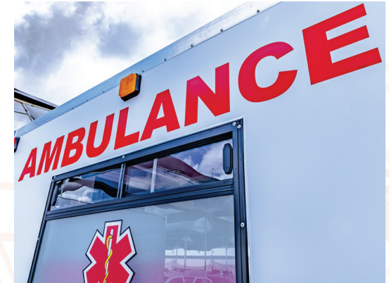
AMBULANCE DECALS AND SLIDING WINDOWS WITH 4MM TOUGHENED FROSTED ARMOUR PLATE GLASS
